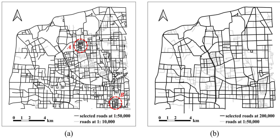
Figure 12. Road network selection results by the proposed method of (a) at the target scale of 1:50,000, and (b) at the target scale of 1:200,000.
