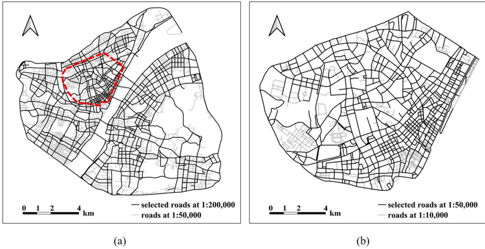
Figure 16. Road network selection results in Wuhan using the models trained in Beijing of (a) at the target scale of 1:200,000, and (b) at the target scale of 1:50,000.
