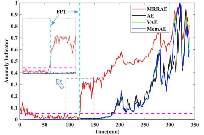
Fig. 8. Anomaly indicator of the XJTU-SY bearing data set.
