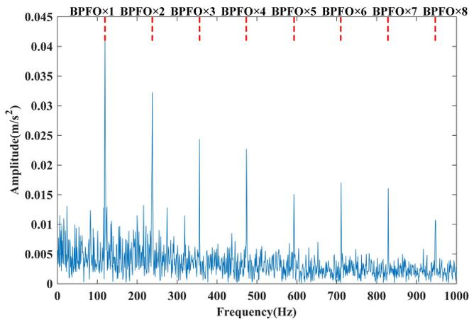
Fig. 10. Envelope spectrum of sensitive band I.
