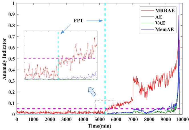
Fig. 5. Anomaly indicator of the IMS bearing data set.
