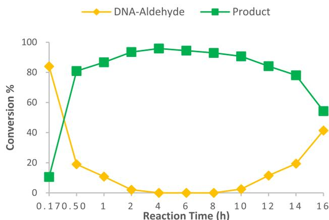
**Figure 4.** Time course studies of the MBH reaction. DNA-aldehyde (**1a**, 0.33 mM), DABCO (1.33 M), olefin (**2**, 0.33 M),  $\text{CH}_3\text{CN}/\text{H}_2\text{O} = 2/1$ , 25 °C, 0 to 16 h.
