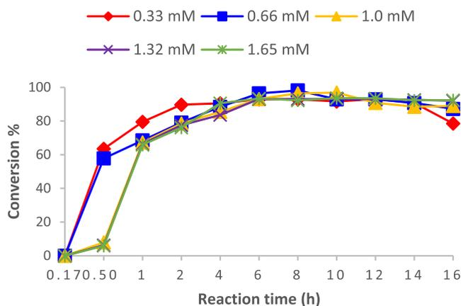
**Figure 2.** MBH reaction of **2** with various concentration of **1a**. DNA-aldehyde (0.33–1.65 mM), DABCO (0.33 M), olefin (0.33 M),  $\text{CH}_3\text{CN}/\text{H}_2\text{O} = 2/1$ , 25 °C, 16 h.
