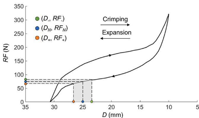
**Fig. 6.** Radial force ( $RF$ ) vs. diameter ( $D$ ) curve obtained from the FE analyses of radial crimping test of the stent-graft, incorporating the material parameters of NiTi wire sample 1. The values of  $RF$ ,  $RF_N$  and  $RF_+$ , corresponding to  $D$ ,  $D_N$  and  $D_+$ , respectively, are represented.
