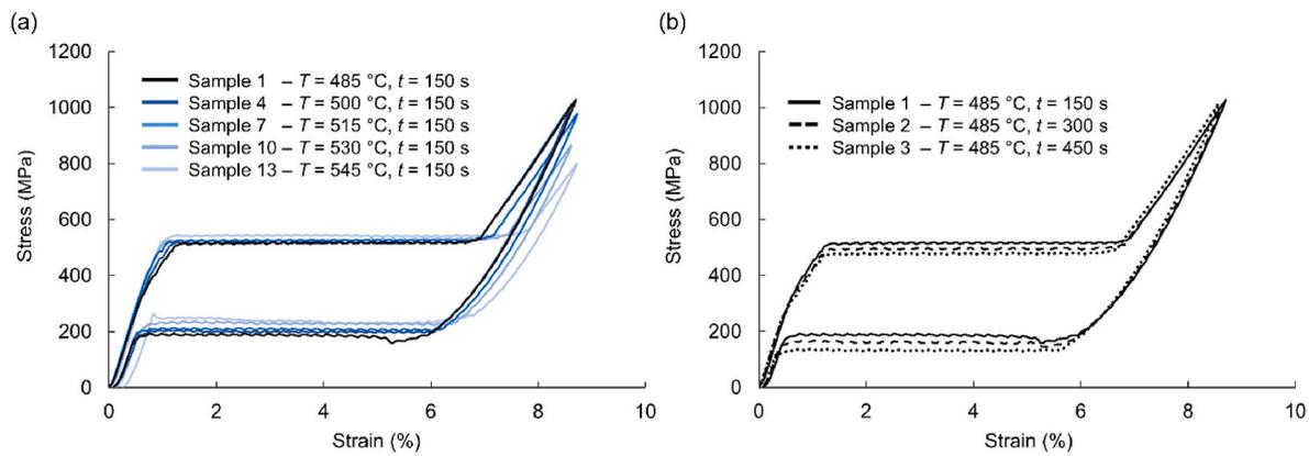
**Fig. 5.** Uniaxial tensile stress vs. strain curve of (a) five NiTi wire samples varying temperature ( $T$ ) and fixing time ( $t$ ); (b) three NiTi wire samples varying  $t$  and fixing  $T$ . Only cycle 2 is shown for all NiTi wire samples.
